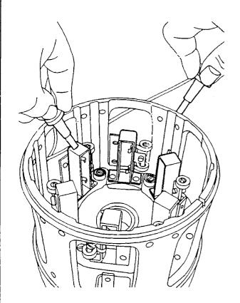
CHECKING/REPLACING CARBON BRUSHES
